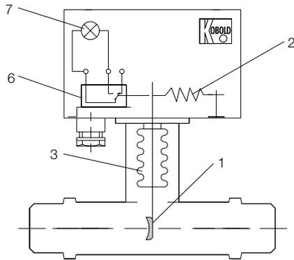
The motion is transferred positively from the baffle (1) to the measuring section.
