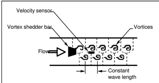
The measuring principle is based on the Karman Vortice Street. A specially shaped bluff body is located in direction of the flow. From a certain flow velocity on vortices are generated through the bluff body. These small vortices generate small pressure differences which are sensed from a piezoelectric sensor behind. The number of vortices is directly proportional to the flow velocity and will be provided to an evaluating electronic.
