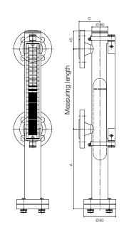
NBK-M... with roller-type display and magnetostrictive transmitter
