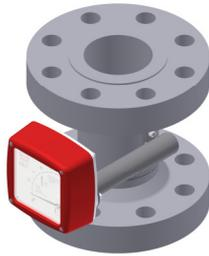
Through the unique structure of the measuring fitting with cylindrical measuring pipe and concial float, the units can be produced with thick walled pipes. This enables the use in high pressure applications for which other measuring instruments are not available e.g. sour gas, tunnel drill machine lubrication
